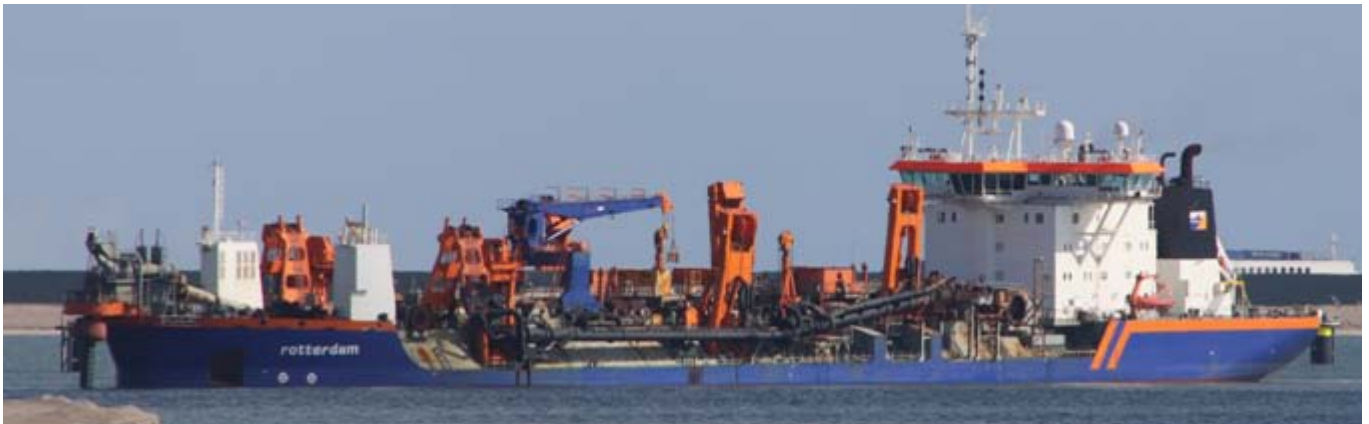
Van Oord's TSHD ROTTERDAM seen pumping the sand towards the beach at Rotterdam-Maasvlakte Photo : Arie Boer (c)
